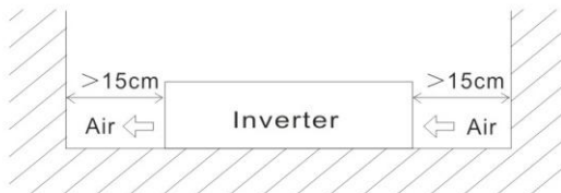
Figure 4.3: Example of Installation
